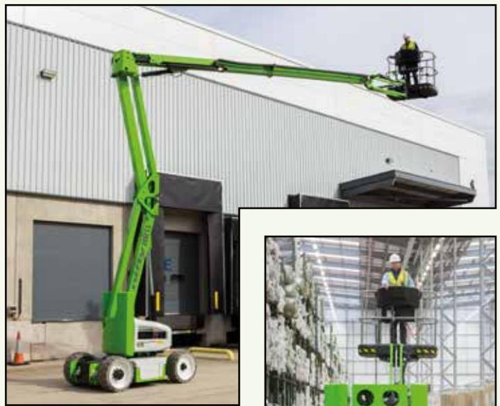
The HR15N's **1.5m width** and **sub 2m height** enables travel through restricted spaces. Optional non-marking tyres mean that it can work both inside and out making it ideal for industrial or maintenance work.
